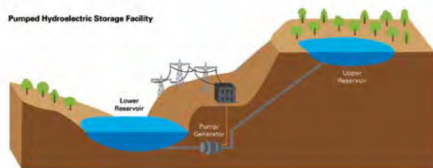
Pumped storage can be thought of as a giant rechargeable battery — pumping water uphill when there's extra energy being produced, and letting it flow downhill to generate energy when needed. Image courtesy of Dominion Energy
