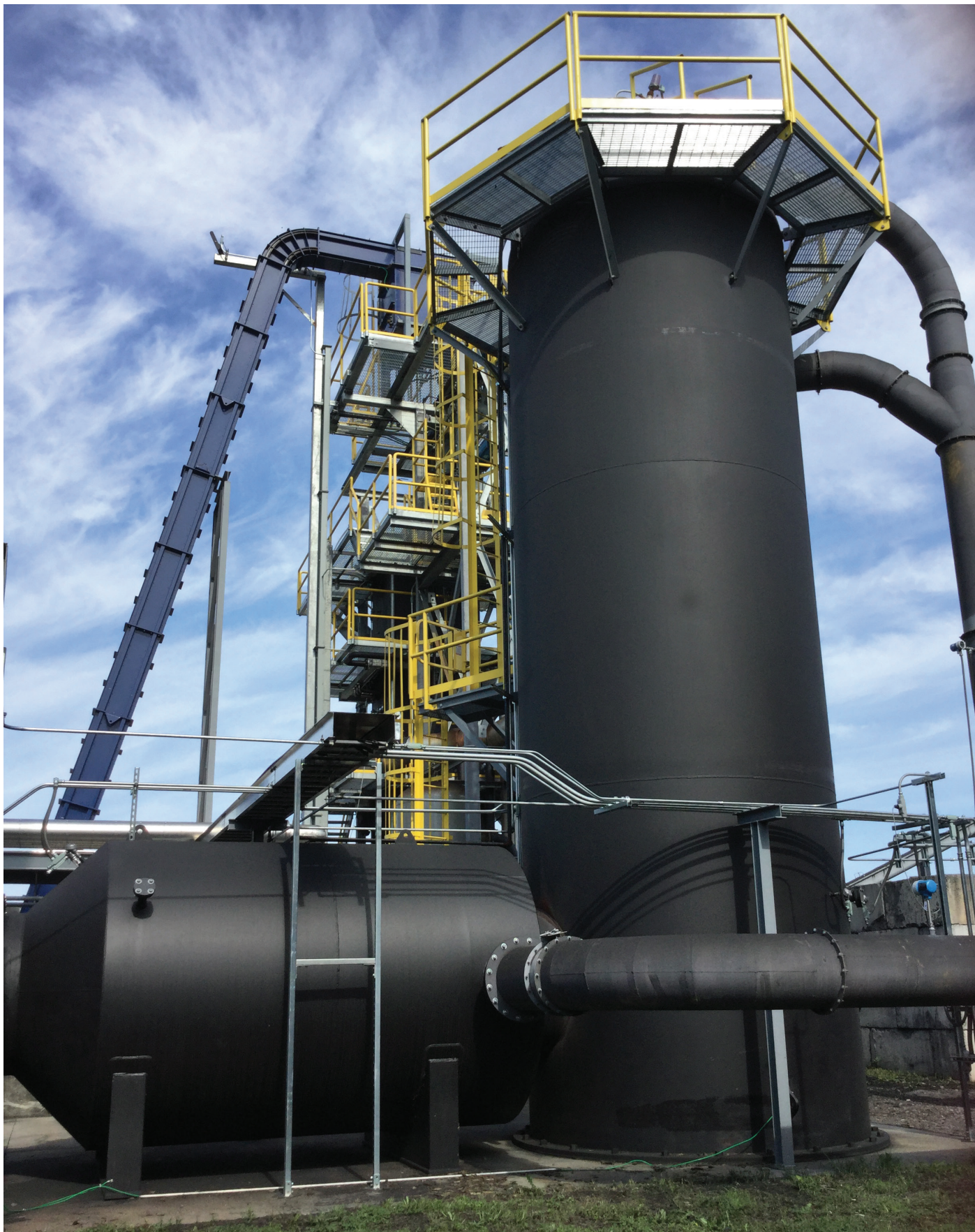
Syngas produced from the gasifier is combusted in an industrial thermal oxidizer, an emissions control device. (photo credit: Dillon Fuller)
