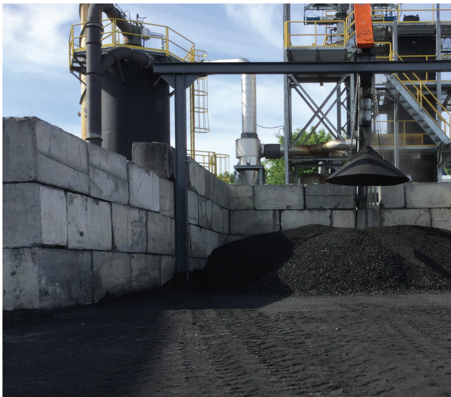
Biochar is the carbon-rich product that is left over after the completion of the gasification process. (photo credit: Dillon Fuller)
