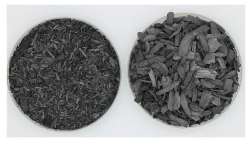
Switchgrass biochar (left) and hardwood biochar (right), both produced at approximately 1,000 C.
